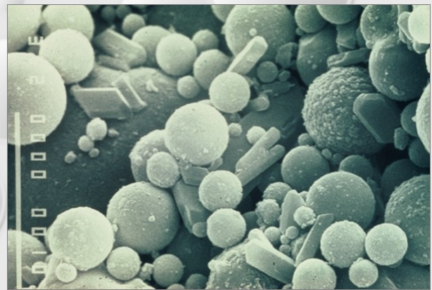
Figure 2 - PFA particles are spherical - giving them some unique properties
