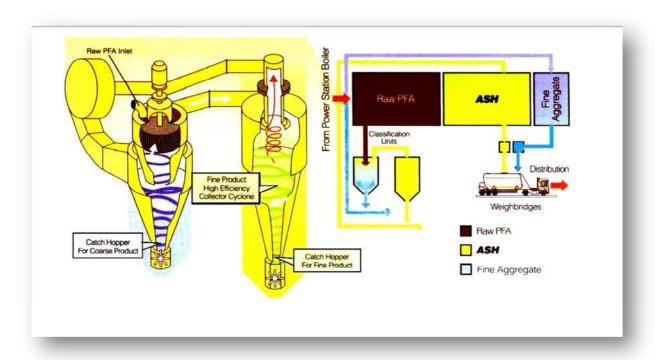
This has been carried out in the UK since the late 1970's and is well established. The air swept classifiers remove coarser ash particles to produce a finer product thereby improving the reactivity in concrete/cement. An alternative or supplement to classification is selection, where ashes are preferentially extracted from the banks of precipitators or the ash output is continually monitored for LOI and when within preset parameters is diverted to a low LOI silo.
