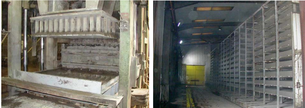
Figure 8 – Static concrete block forming machine (left) and curing kiln (right)
