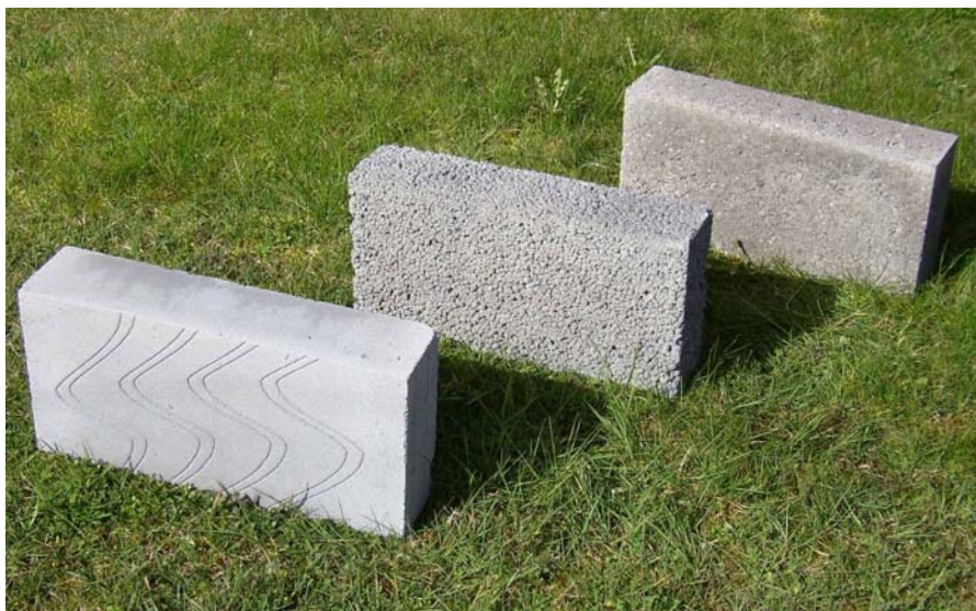
Figure 1 - Aerated (front), lightweight aggregate (middle) and dense aggregate (back) concrete masonry units
