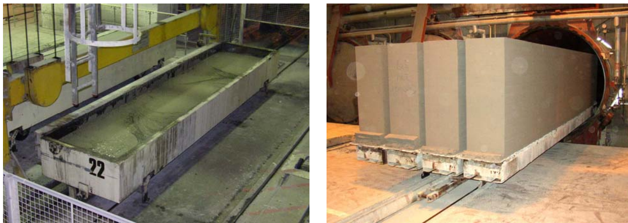
Figure 7 - Casting (left) and autoclaving (right) of AAC
