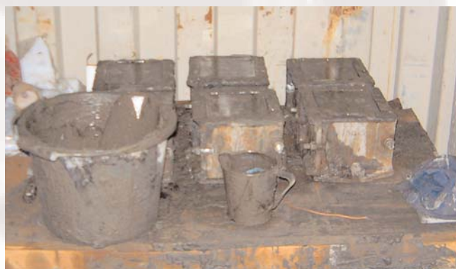
Figure 4 - Taking test cubes
