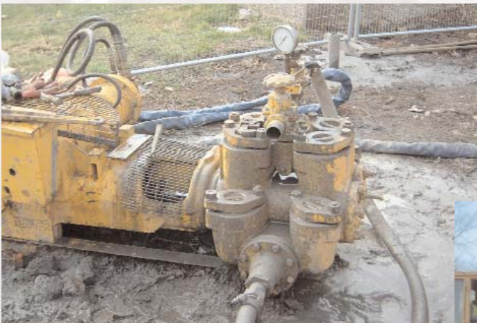
Figure 6 - A hydraulically powered, piston type grout pump
